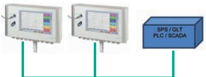
RS 485 Network (Modbus RTU) oder Ethernet (Modbus/TCP)
